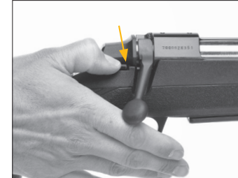
Press the bolt lock override button and lift the bolt handle.
